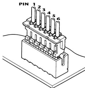
Sensored type compatible speed controls must use the six position JST header part number X-6B-ZRSMX-TK (where X denotes the style of the header) or equivalent. The power motor wire connections must be clearly marked A, B, C on both speed control and motor. A for phase A; B for phase B; C for phase C
